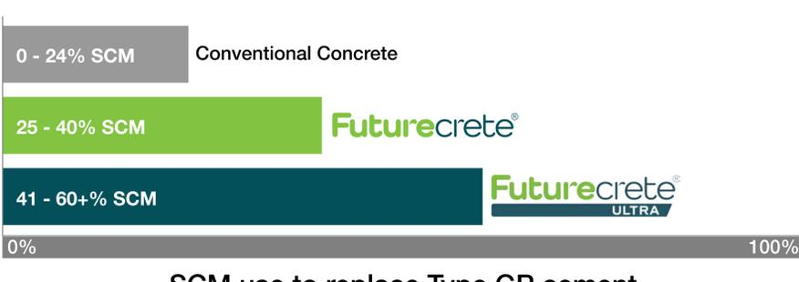
Supplementary Cementitious Materials (SCMs) are re-purposed industrial by-products which possess cementing properties but have much lower embodied carbon. By replacing a portion of cement with SCMs in concrete, the embodied carbon of the mix can be lowered. Futurecrete<sup>®</sup> uses a minimum of 25% SCMs to save on carbon. Futurecrete<sup>®</sup> Ultra uses a minimum of 41% SCMs.
